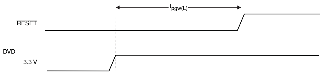
Figure 34. Reset Timing During Power On
